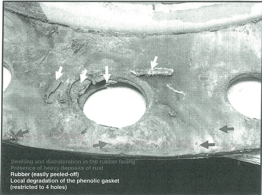
FIGURE # 12 Portions of rubber facing torn apart during dismantling.
